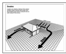
R - The grading should be improved to promote the flow of storm water away from the house and off the lot. The ground should slope away from the house at a rate of one inch per foot for at least the first ten feet. Ideally, at least eight (8) inches of clearance should be maintained between soil level and the top of the foundation walls. See comments/recommendations under foundations. Trenching, against the foundation, is not acceptable.
